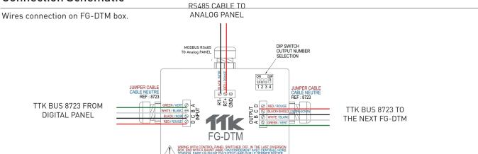
Wires connection and loop on the last FG-DTM box on a circuit.
