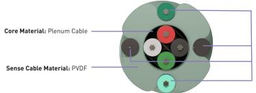
Four Sensor Wires Material: PVDF
